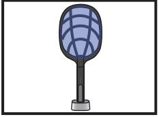
2. The Magic Mesh ™ bug zapper will glow blue, and the high voltage will be on constantly without holding down the high voltage button. WARNING: At this point, do not touch the metal mesh!
