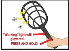
2. Press and hold the high voltage button switch. The red high voltage will turn on and the product is ready to use.
