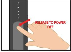
3. Once the high voltage button is released, the high voltage function turns off.
